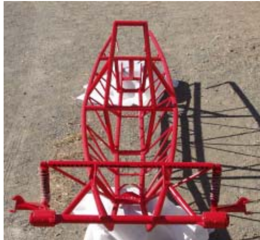
Prototype spaceframe chassis of the EV.
